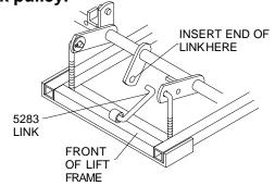
2. Remove front and rear deck hanger pins, as illustrated below.
